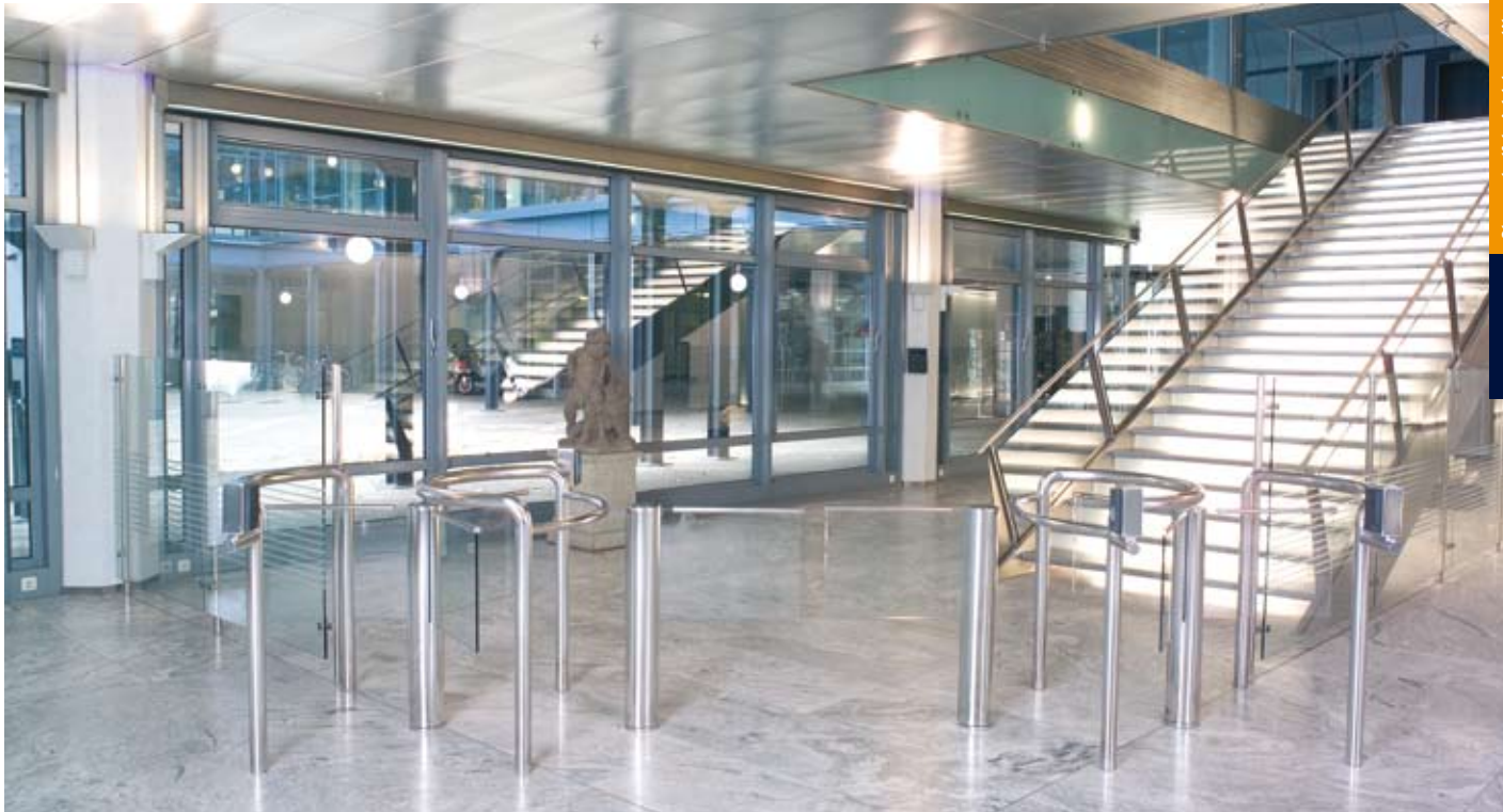
Charon HTS-E03 half-height turnstiles and HSD-E03 swing doors
